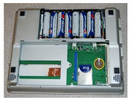
hile most laptops and netbooks use expensive proprietary battery packs that wear out and need to be replaced, the Gecko Edubook uses standard, low-cost AA NiMH batteries. The Gecko Edubook will run for 4 hours per charge with 2000 maH batteries.
